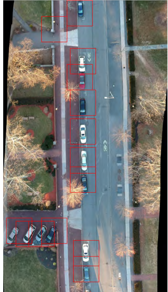
Figure 14: An example of our car classifier using Version 2 of our net. This generated 0 false negatives and 1 false positive
