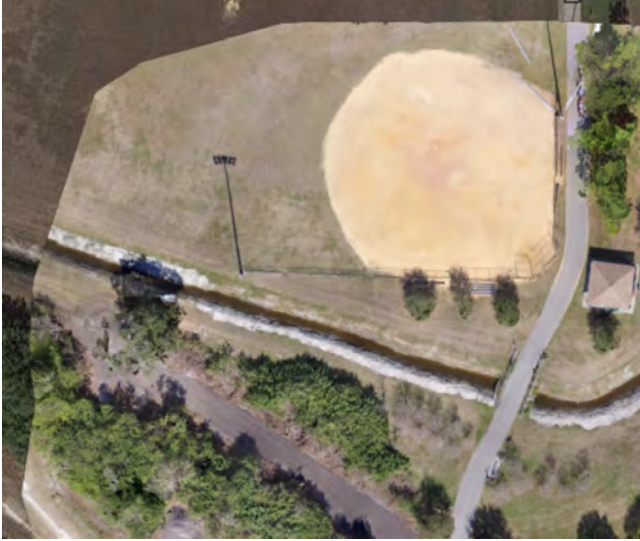
Figure 1: Sample map output from 3DR Site Scan, with evident warping and stitching present
